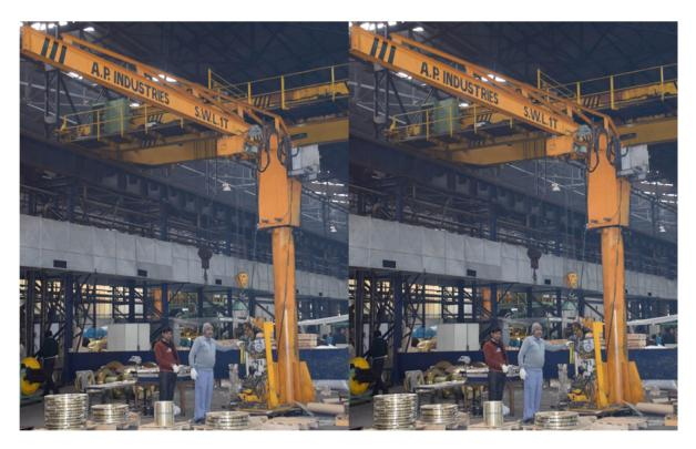
Column mounted Jib Cranes are necessary when no other appropriate support near a workstation is available. The Jib arm of this type is attached to steel pipe swivelling on antifriction bearings. Wall mounted Jib Cranes are ideal solutions for workstations located near walls or vertical structures. The Jib arm of these type are mounted on building column made from steel. Special design is also available for mounting of Jib arm on RCC columns.
